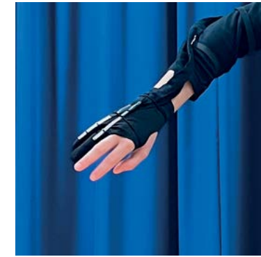
Fig.21: Testing the glove (flex sensors) that control the airflow around the hips
